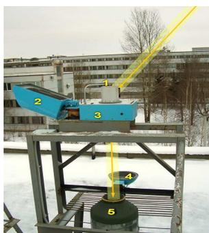
Fig. 2 Original sun-tracker system (on the roof) for Bruker IFS125 HR designed at the Dept. of Atmospheric Physics.
