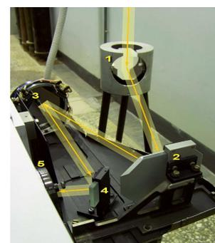
Fig. 3 Original sun-tracker system for Bruker IFS125 HR designed at the Dept. of Atmospheric Physics.
