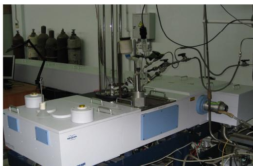
Fig. 1 Fourier spectrometer Bruker IFS125 HR.
